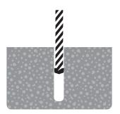
1. **Drilling** Use drill in hammer mode. Drill to specified diameter and depth for the required size.
