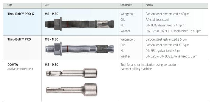
\* Sherardising is a process of galvanisation of ferrous metal surfaces, also called dry galvanising. The process involves heating the steel up to 500°C in a closed rotating drum that contains metallic zinc dust.
